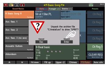
The installation data is now available on the stick and can be installed as described below. **But first a tip**: Delete the archive file again from your factory data stick after installing the data. Otherwise, the display will always ask whether the file should be unpacked when you insert the stick into the organ, since archive files are automatically recognized. The unpacking has now already been done and the archive file can thus be deleted from the stick, it is no longer needed.
